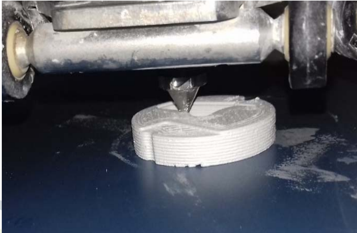
Formulation S_PVA_OA_9 (alumina D=0.4\mu\text{m} ) printing a gas dosing valve disc
